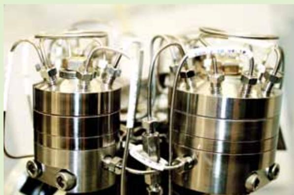
The 700XA gas chromatograph has the capacity to support up to four 10-port or 6-port diaphragm/piston valves, which are guaranteed for the life of the system.
