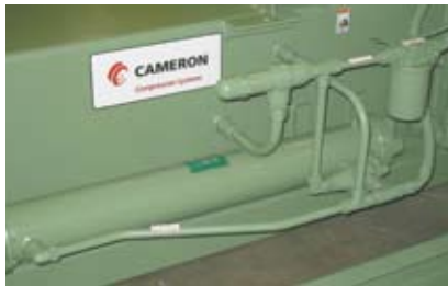
Self contained, low pressure lubrication system.
