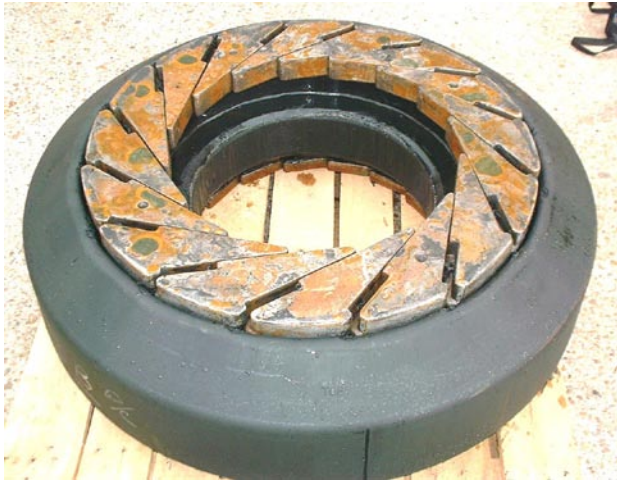
18-3/4"-5000 psi D/DL Annular Packing Element Subassembly After Cold Test
