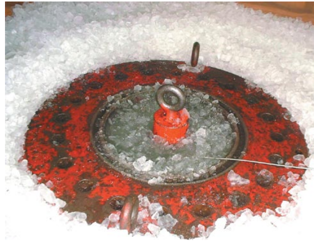
18-3/4"-5000 psi D/DL Annular BOP In Ice Prior to Cold Test
