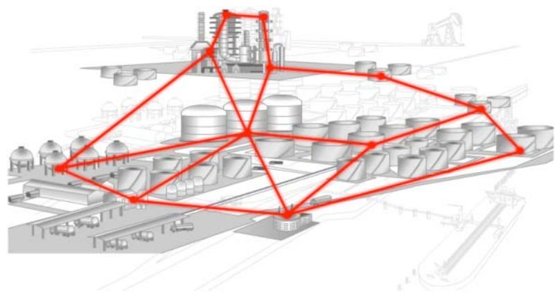
Figure 3. A wireless site survey addressed the coverage area desired at the Gallup refinery, existing power and network infrastructure, and interfering and operating frequencies currently in use or ambient in the environment.
