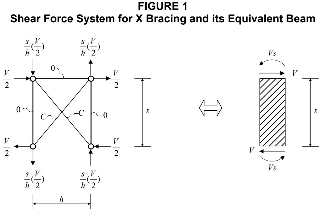
The forces in the diagonals are  $\pm C = \pm(V/2)d/h$ , where  $d$  is the diagonal length, and the corresponding complementary energy for the 2D lattice truss is:
