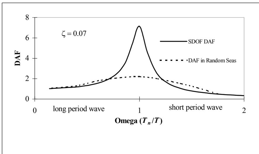
Care should be taken when determining the appropriate wave period to be used in an SDOF analysis. A range of wave periods should be investigated, along with a range of associated wave heights. The applicable sea states that result in maximum responses should be identified and used in the assessment of the adequacy of the structure's strength.
