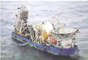
**The reel-lay vessel Norlift transferred from the North Sea to lay 6- and 8-inch lines, to tie back deep water wells on the Zafiro field.**
