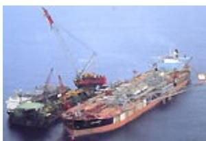
**DLB Polaris lifting a total of 12,000t of process modules, for boosting the Zafiro producers capacity to 80,000b/d.**
