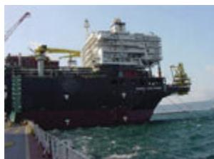
**The Sanha LPG FPSO has an LPG storage capacity of 135,000m<sup>3</sup> in six tanks and a daily processing capacity 6,000m<sup>3</sup>.**
