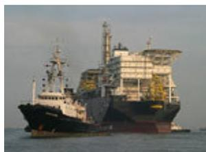
**The Sanha LPG FPSO is the first floating production facility to combine all LPG processing and export functions onboard the same unit.**
