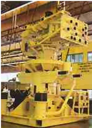
**The ANM subsea christmas tree, capable of bearing substantial pressure 2,000m under the sea.**
