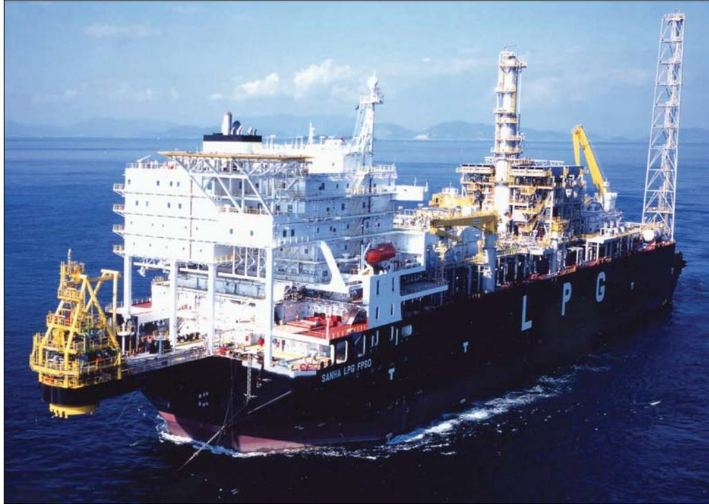
In selecting a tanker for FPSO conversion, hull girder strength as well as yielding, buckling and fatigue of primary and secondary structure must be verified\*
