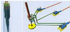
**A CAD detail of the top of the riser tower (left) and the riser tower on the seabed (right).**
