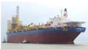
**The FPSO is moored to the seabed by 32t anchors, connected to the turret by ten chain/polyester rope lines.**
