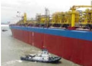
**The FPSO topsides process system was designed by Gusto, which based the layout on 17 separate modules, located along a central piperack system.**
