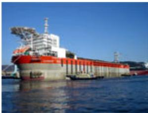
**The Greater Plutonio accumulation lies in 1,200m to 1,500m of water. Its development involves the use of subsea wells tied back to a single spread moored FPSO facility.**
