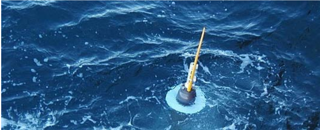
ARGO Float – image courtesy of Sabrina Speich
